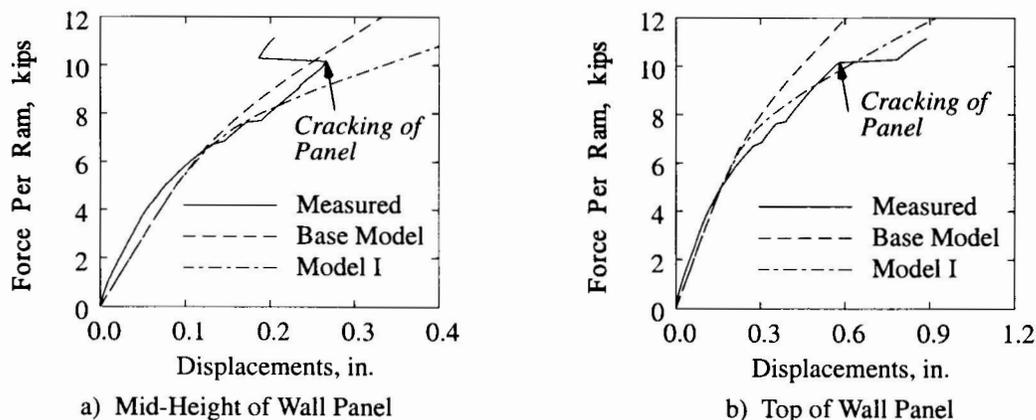
Fig. 4 Modified Measured and Calculated Out-of-Plane Displacements of the Longitudinal Wall Panel
