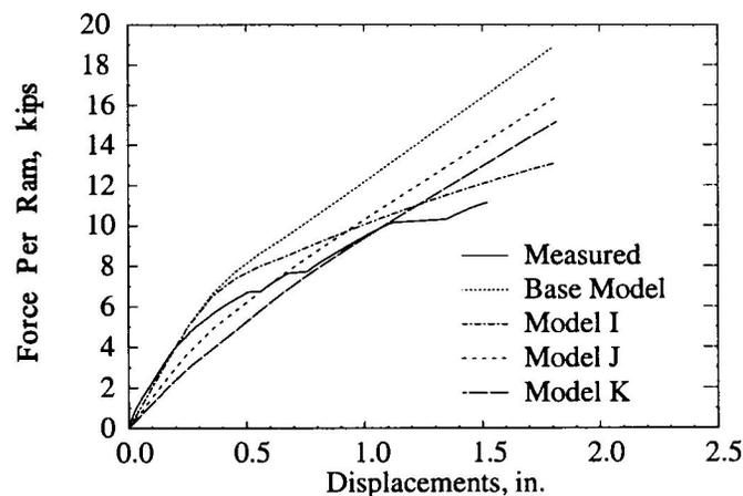
Fig. 3 Calculated Transverse Displacement at Midspan of the Diaphragm TU1
