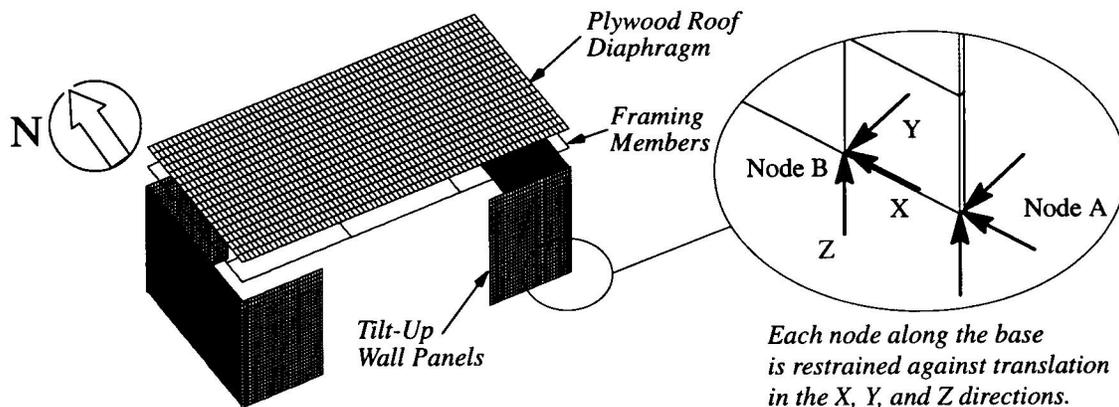
Fig. 2 F.E. Model of Specimen TU1 and the Boundary Conditions for the Base of the Wall Panels
