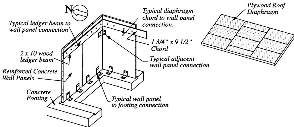
Fig. 1 Schematic View of Structural Components of Specimen TU1
